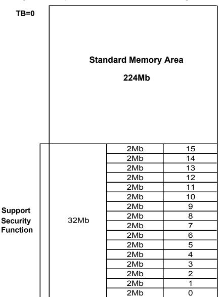
Figure 4: Example of how ArmorFlash could be configured
